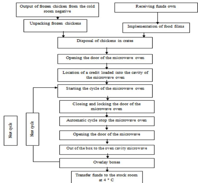
Figure 1. Diagram of thawing in the microwave oven
